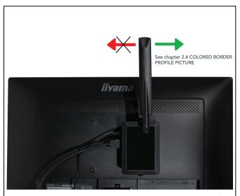
Check the connection status. A led on the top of the media player indicates the connection status. **Green**: your Spiqle is connected to the internet successfully. **Red**: There is no connection. Try to improve the connection by turning the antenna clockwise (seen from behind). Reboot the media player to restart the connection See chapter **2.4 COLORED BORDER PROFILE PICTURE**
