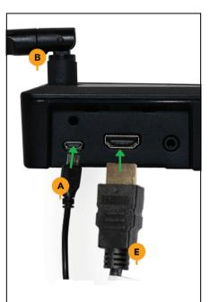
Connect the HDMI cable (E) and the power supply (A) to the media player (B)
