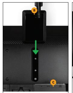
Keep the media player (B) above the two screws pointing out of the bracket on the rear part of the display (C). Now, slide the media player down to attach it to the mounting bracket
