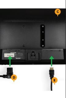
Connect the power cord (D), the HDMI cable (E) to the display and to the media player Place your Spiqle at the desired location and plug in the power power adapter (A) and the power cord (D) in the wall outlet
