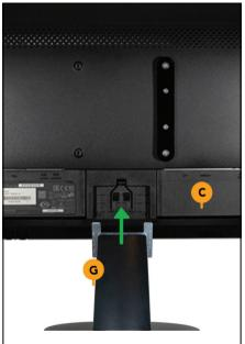
Slide the completed foot (G) in the slot on the back of the monitor (C). Press until you hear it clicking in place
